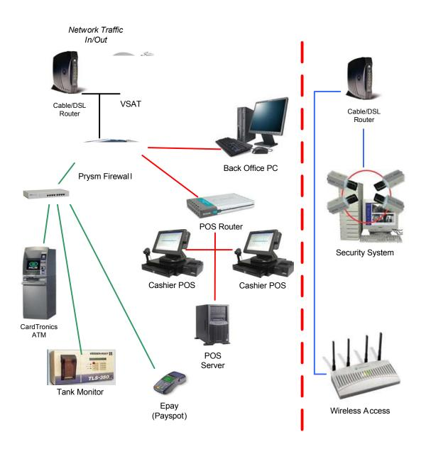
The cable router, the VSAT, or DSL (and the phone line for dial backup) enter the store through the Prysm firewall. The Prysm is a firewall that separates traffic between the Internet, the store's internal LAN, the secure network used to process credit cards, and the vendor network used to maintain your equipment. It is very important that devices be plugged into the proper location on the Prysm, and that other devices are not put between it and the broadband connection.
